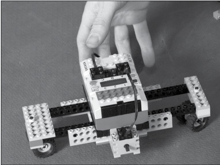
**Figure 1.1** A student-created robot contains a programmable "brick," or processor, in the center.
