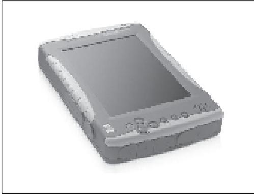
FIGURE 1.2. | A ruggedized slate tablet PC
